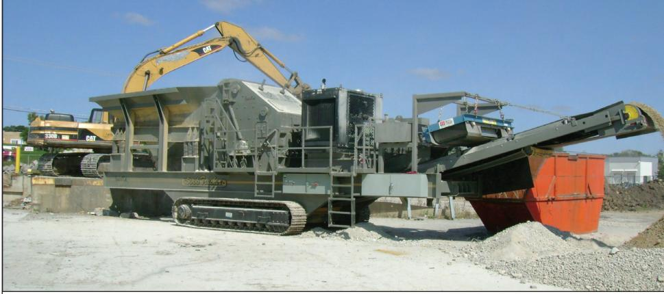
5066 Tracker diesel engine drives crusher, hydraulic pumps for tracks and clutch and generator for all electric motors.
