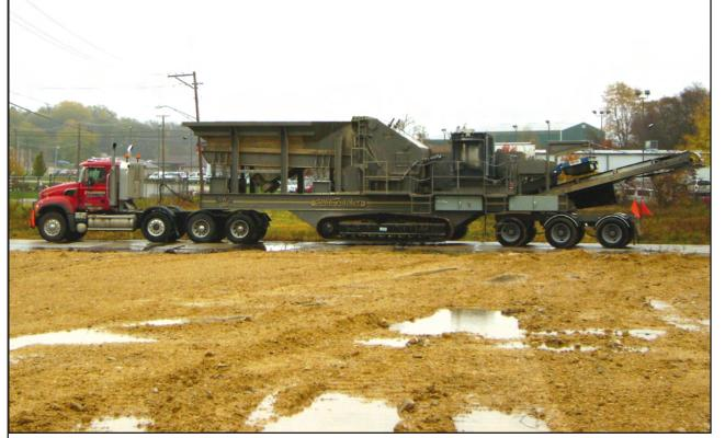
5066 Tracker features quick and easy transport capability using built in three axle bogey.
